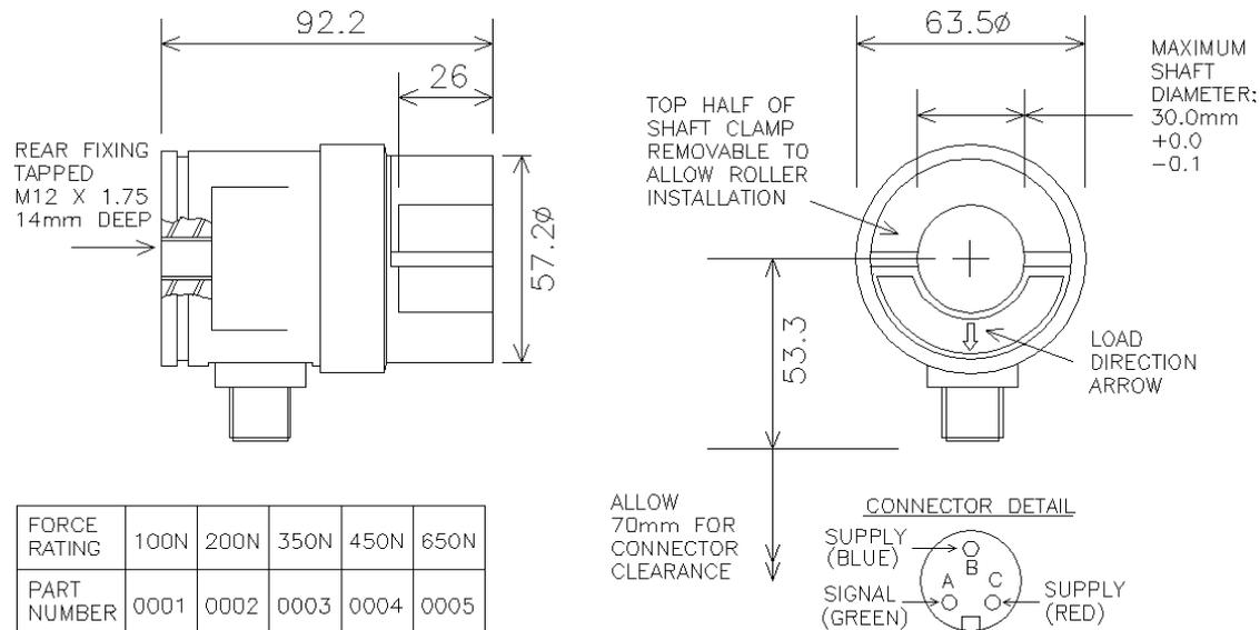
When selecting a transducer mounting location, please remember that the tension sensing roller must **NOT** be mounted where the web wrap angle can vary. Any change in the wrap angle will be sensed by the transducer as a change in tension, and indicated as such on the tension meter or display.
